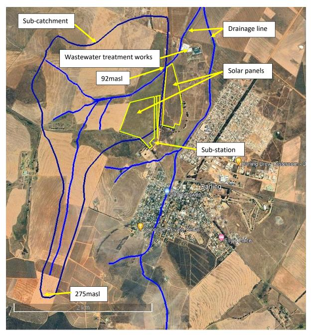
Figure 6 Drainage Lines and Sub-Catchment
