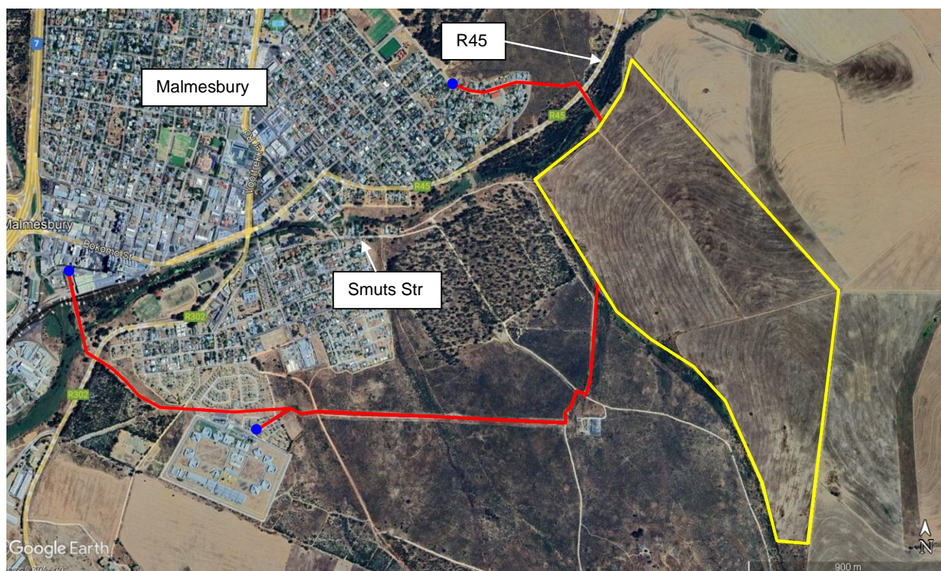
Figure 1: Google Earth image showing the locality of the proposed solar PV site area (~130ha assessed area)(yellow polygon) and the power cable routes (red lines) to the existing sub-stations (blue circles).
