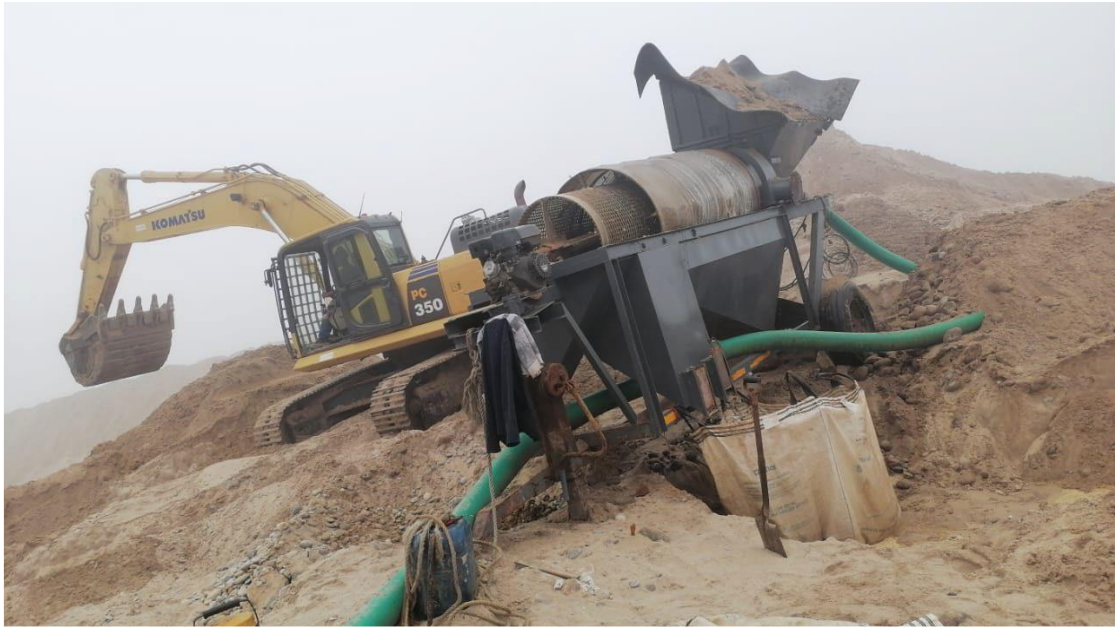
Figure 2-4: Infield trommel screen used to process the mined sediments.
