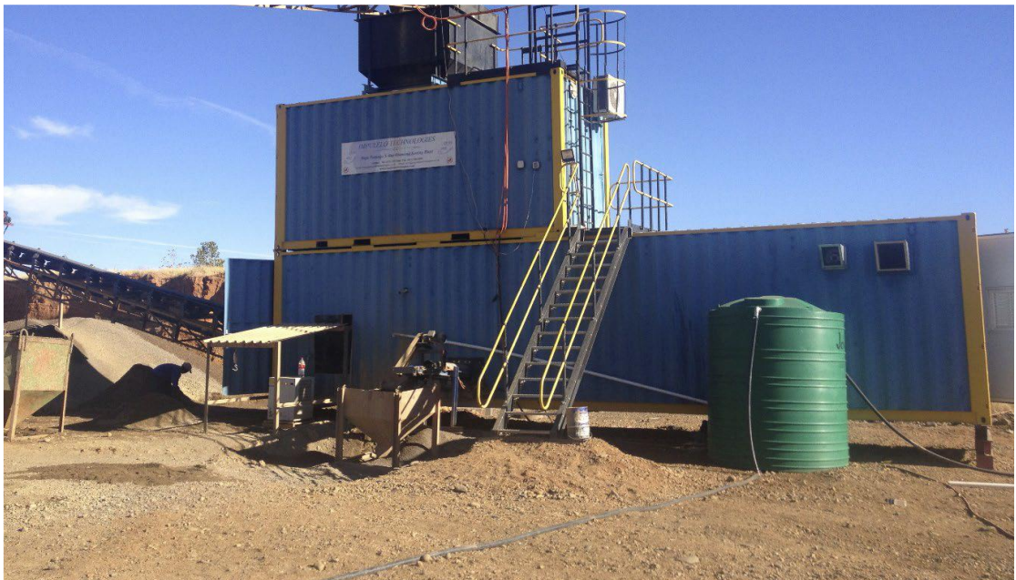
Figure 2-5: Mobile containerised processing plant.
