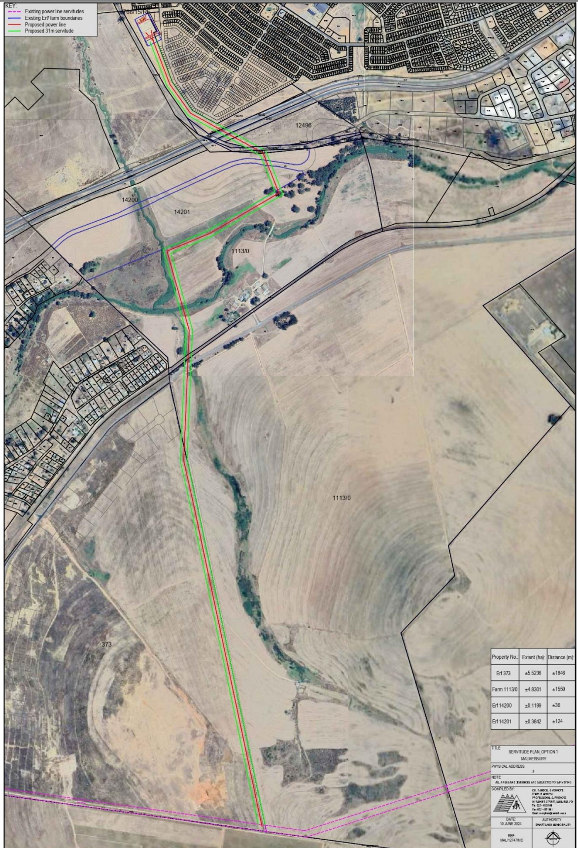
Figure 7: Preferred 132 kV overhead powerline route
