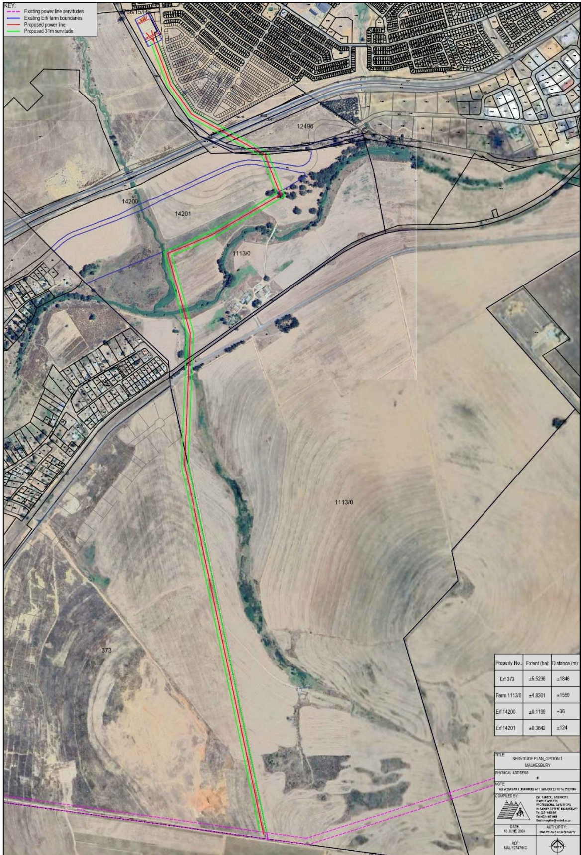
Figure 3: Preferred 132 kV overhead powerline route
