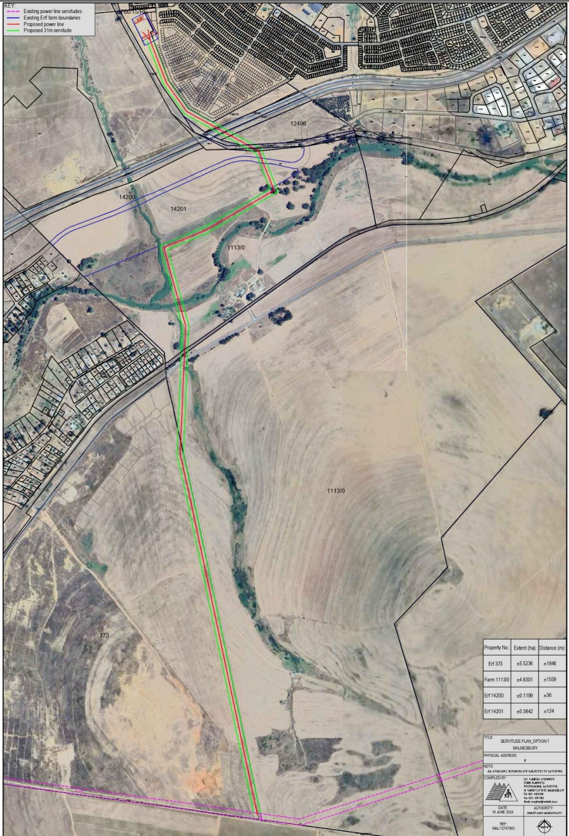
Figure 7: Preferred 132 kV overhead powerline route
