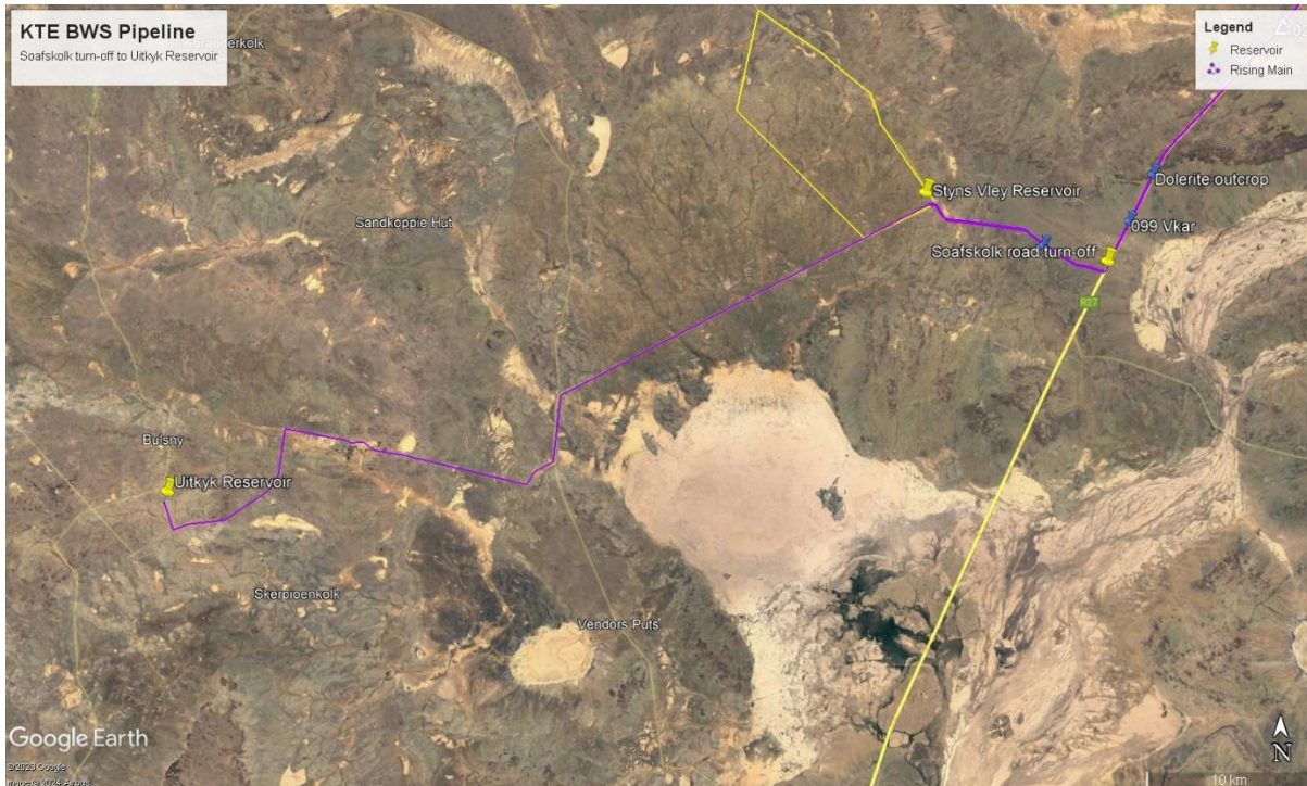
Figure 10: Google Image showing the proposed pipeline route (purple), following secondary farm roads from the Soafskolk turn-off, first to Farm Styns Vley (yellow polygon) and then on to the reservoir on Farm Uitkyk.
