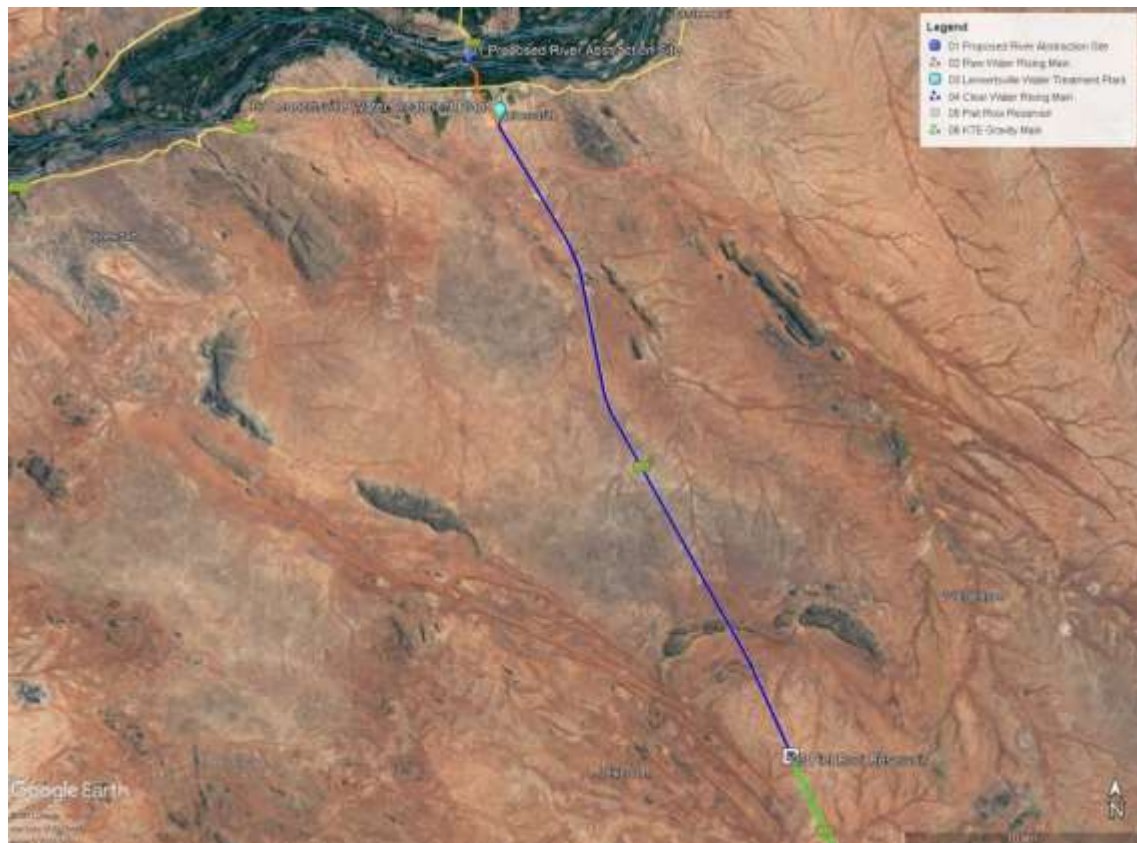
Figure 2. Close up view of the pipeline from the Abstraction point at the Orange River to the Piet Rooi Reservoir.
