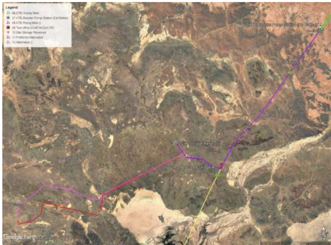
Figure 4. Close up view of the pipeline from the Booster Pump station to the proposed evaporation ponds at the end of the pipeline route.
