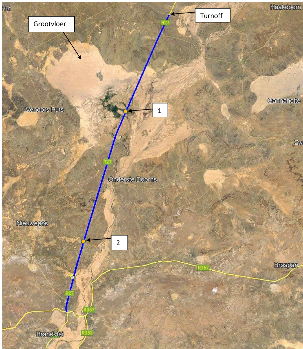
Figure 9 Proposed pipeline from the Turnoff to Brandvlei.
