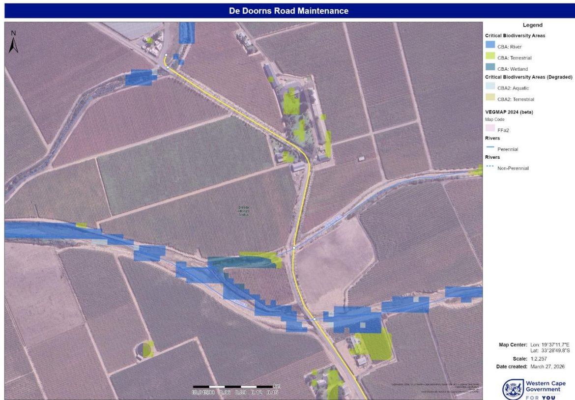
Figure 4: The WCBSP (2023) CBA map showing the DR1489 (yellow) – culverts and bridges (CapeFarmMapper).
